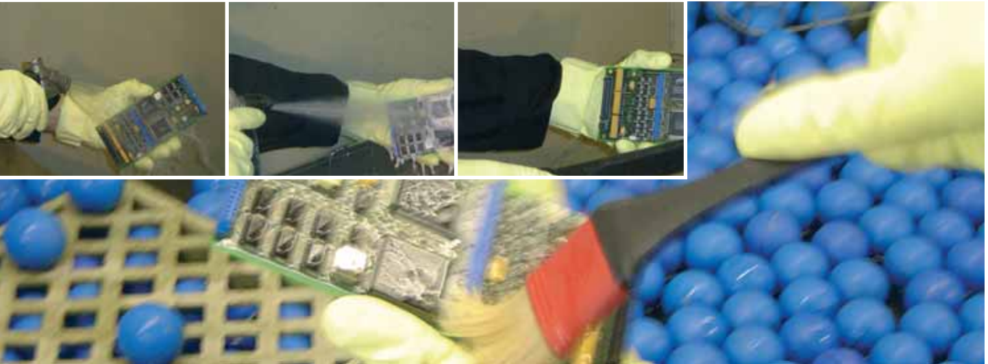
above (large): bath cleaning of printed circuit board above (small): wet cleaning procedures
